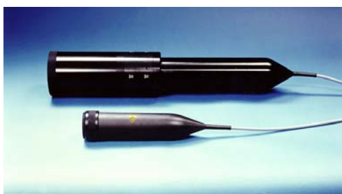
Figure 19. Photograph of modern commercial fiber optic based LDA probes.
