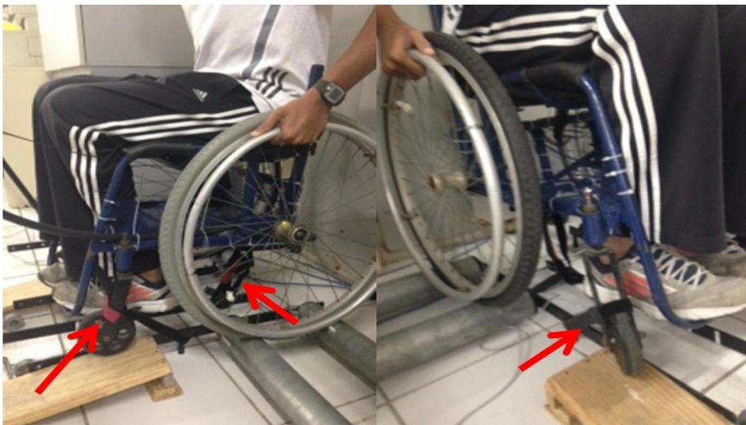
**Figure 2.** Tires of the wheelchair fixed by a roller dynamometer. Red arrows show the belts for lateral movement of the wheelchair.
