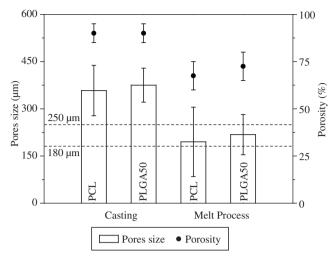
**Figure 3.** Average of pore sizes ( $\mu$ m) and average porosity (%) of PCL and PLGA50 scaffolds prepared by casting and melting compression process.
