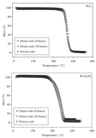
Figure 4. Thermogravimetric analysis of samples of PCL and PLGA50 prepared by melting compression process.
