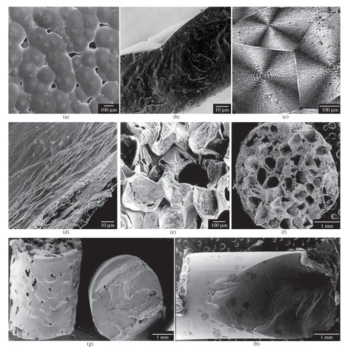
Figure 2. Scanning electron micrographs of PCL and PLGA50 scaffolds. a) and b) dense PCL membranes; c) Optic microscopy of PCL membranes; d) PLGA50 dense membranes; e) PCL porous membranes; f) PLGA50 porous rods; g) PCL porous (left) and dense (right) rods and h) PLGA50 dense rods.
