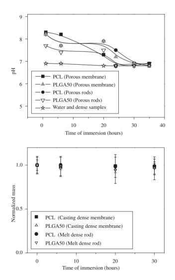
Figure 1. Normalized mass and pH variation of PCL and PLGA50 samples in distilled water.
