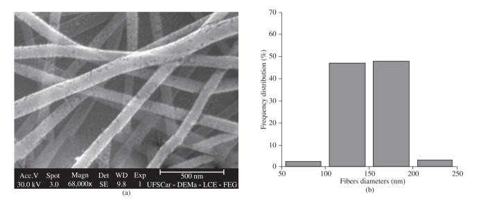
Figure 5. a) Micrograph of sample F 13 (Phillips® SEM); and b) diameter distribution (Zeiss® SEM).
