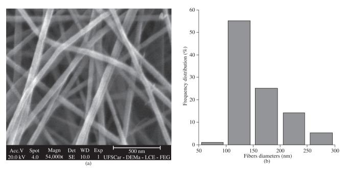
Figure 7. a) Micrograph of sample DS6 (Phillips® SEM); and b) diameter distribution (Zeiss® SEM).
