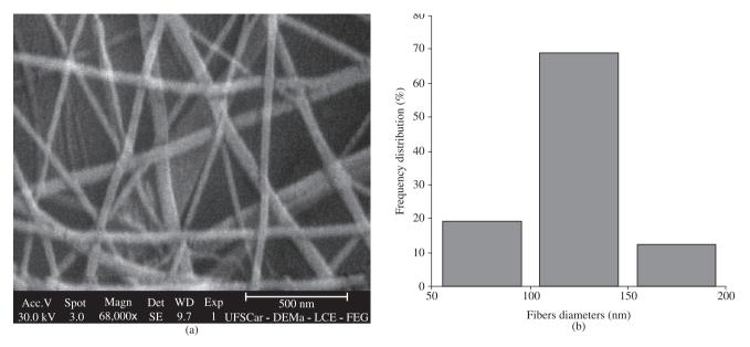
Figure 2. a) Micrograph of sample A5 (Phillips® SEM); and b) diameter distribution (Zeiss® SEM).
