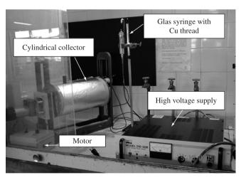
Figure 1. Electrospinning set-up used in this work.
