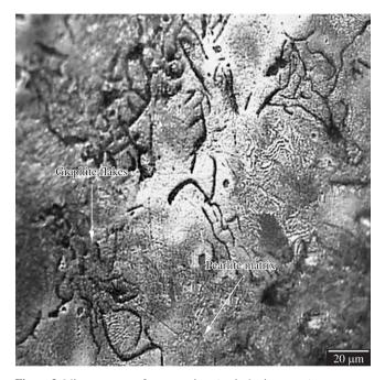
Figure 3. Microstructure of gray cast iron (optical microscope).
