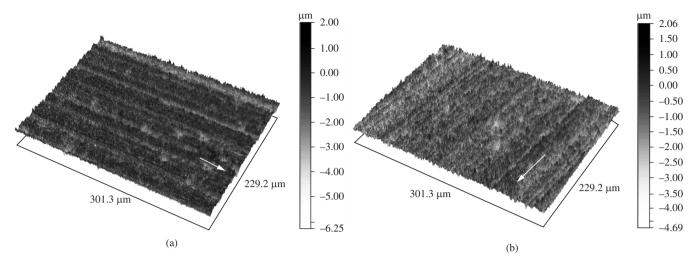
**Figure 5.** Optical profiler images of a  $\beta$ -Si<sub>2</sub>N<sub>4</sub> cutting tool: a) grounded, and b) AlCrN coated.
