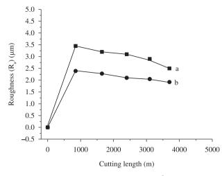
Figure 7. Workpiece roughness vs. cutting length, for  $\beta$ -Si<sub>3</sub>N<sub>4</sub>: a = uncoated; and b = AlCrN coated.
