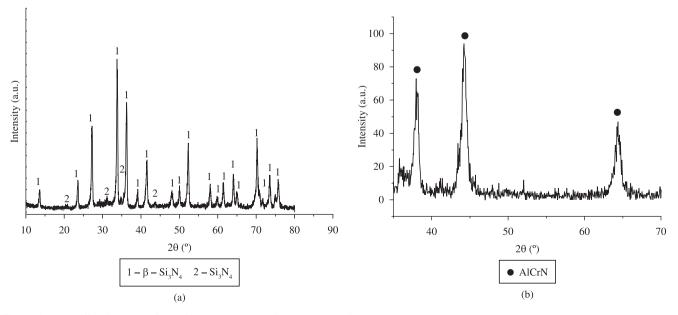
Figure 4. X-ray diffraction pattern for: a)  $Si_3N_4$  tool; and b) AlCrN coated tool (GIXRD).
