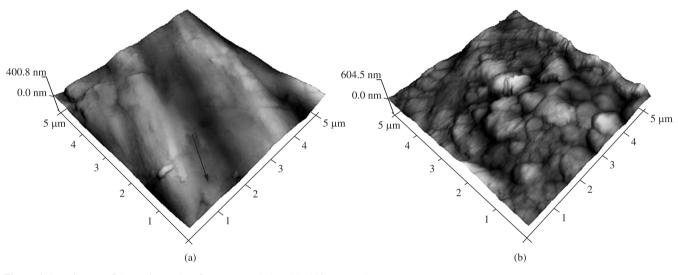
Figure 6. AFM images of the cutting tool surface: a) grounded, and b) AlCrN coated.
