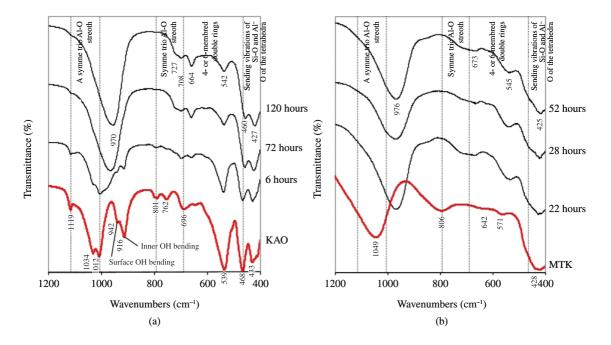
Figure 9. FTIR spectra of unreacted raw materials and the as-synthesized zeotypes obtained after hydrothermal transformation of (a) kaolinite and (b) metakaolinite in 1.33 M NaOH solutions at 100 °C after several reaction times.
