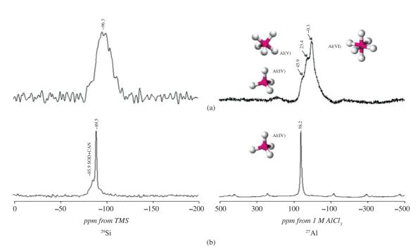
Figure 11. <sup>29</sup>Si and <sup>27</sup>Al MAS-NMR spectra of the (a) starting metakaolinite and (b) representative as-synthesized zeotypes obtained after hydrothermal transformation of metakaolinite in 1.33 M NaOH solutions at 100 °C after 52 hours of reaction.
