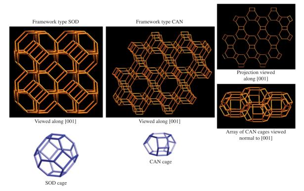
Figure 1. Framework structures of SOD and CAN, showing their characteristic cages and channels, adopted and modified from the Database of Zeolite Structures<sup>7</sup>.
