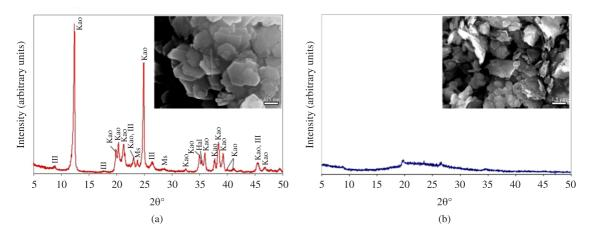
Figure 2. X-ray diffraction patterns and SEM images of the starting materials (a) kaolinite and (b) metakaolinite. Kao, Kaolinite; Ili, illite; Ms, muscovite; Hal, halloysite.
