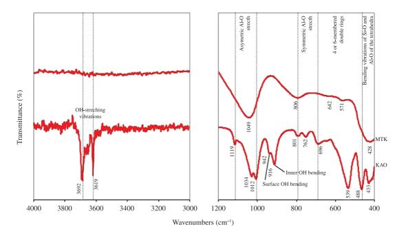
Figure 3. FTIR spectra of the starting materials. KAO, kaolinite; MTK, metakaolinite.
