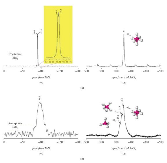
Figure 4. Soli-state <sup>29</sup>Si and <sup>27</sup>Al MAS-NMR spectra of the starting materials: (a) kaolinite and (b) metakaolinite.
