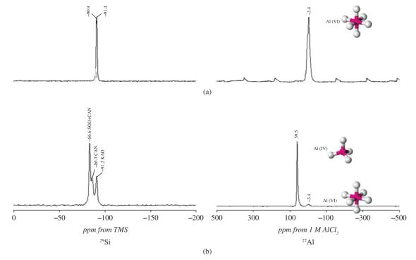
Figure 10. <sup>29</sup>Si and <sup>27</sup>Al MAS-NMR spectra of the (a) starting kaolinite and (b) representative as-synthesized zeotypes obtained after hydrothermal transformation of kaolinite in 1.33 M NaOH solutions at 100 °C after 120 hours of reaction.
