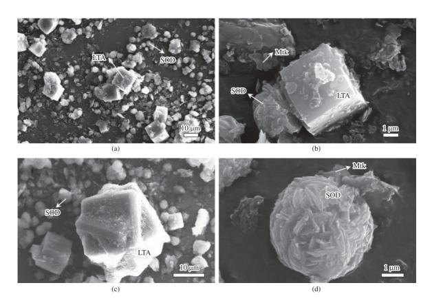
Figure 8. SEM images showing several synthesis products obtained by hydrothermal treatment of the starting metakaolinite in (a)(d) 1.33 M NaOH solutions, after 52 hours of reaction at 100  $^{\circ}$ C.
