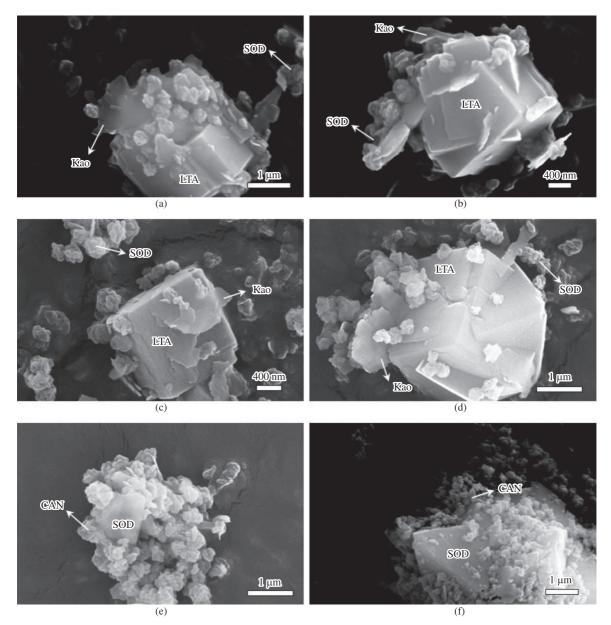
**Figure 7.** SEM images showing several synthesis products obtained by hydrothermal treatment of the starting kaolinite in (a)(b) 1.33 M NaOH solutions, after 6 hours of reaction at 100 °C, (c)(e) 1.33 M NaOH solutions, after 120 hours of reaction at 100 °C, and (f) 3.99 M NaOH solutions, after 120 hours of reaction at 100 °C.
