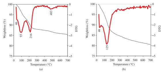
Figure 12. TG/DTG curves from 25 to 700  $^{\circ}$ C of the representative as-synthesized zeotypes obtained after hydrothermal transformation of (a) kaolinite and (b) metakaolinite in 1.33 M NaOH solutions at 100  $^{\circ}$ C after 120 hours and 52 hours of reaction, respectively.
