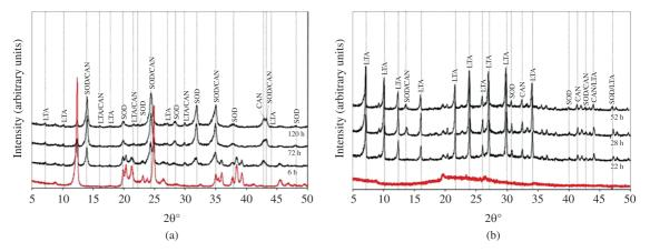
Figure 6. X-ray diffraction patterns of the as-synthesized zeotypes after reaction of the starting (a) kaolinite and (b) metakaolinite in 1.33 M NaOH solutions at 100  $^{\circ}$ C for several times.
