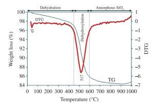
Figure 5. TG/DTG curves between 25-1000 °C for kaolinite.
