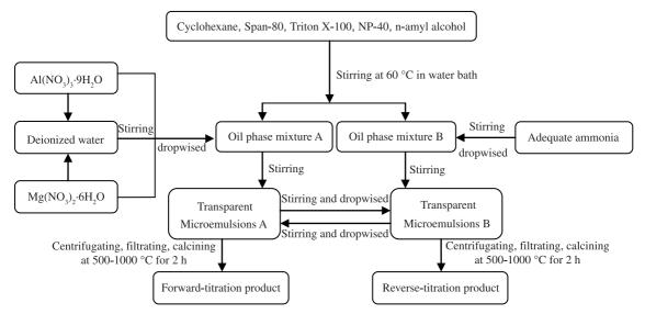
Figure 1. Schematic diagram of synthesize of MgAl<sub>2</sub>O<sub>4</sub> nanoparticles by reverse microemulsion method.
