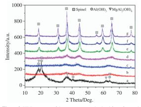
**Figure 3.** XRD patterns of the precursor synthesized from forwardtitration process and powders calcined at different temperatures for 2h (a. as-prepared; b. 500 °C; c. 600 °C; d. 700 °C; e. 800 °C; f. 900 °C; g. 1000 °C).
