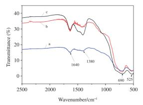
**Figure 6.** FT-IR spectra of  $MgAl_2O_4$  nanoparticles calcined at 900 °C for 2h (a. SPAN-80 + Triton X-100, forward-titration; b. SPAN-80 + Triton X-100, reverse-titration; c. NP-40, forward-titration).
