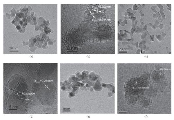
**Figure 5.** HR-TEM images of  $MgAl_2O_4$  nanoparticles calcined at 900 °C for 2h (a,c,e.morphology image of nanoparticles, which synthesized conditions of SPAN-80 + Triton X-100, forward-titration, and SPAN-80 + Triton X-100, reverse-titration, and NP-40, forward-titration, respectively; b, d, f. lattice fringe image of nanoparticles from a, c, e, respectively).
