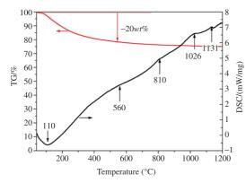
Figure 2. TGA–DSC curves of the precursor synthesized from forward-titration process.
