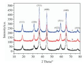
**Figure 4.** X-ray diffraction patterns of  $MgAl_2O_4$  samples calcined at 900 °C for 2h (a. SPAN-80 + Triton X-100, forward-titration; b. SPAN-80 + Triton X-100, reverse-titration; c. NP-40, forwardtitration).
