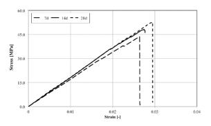
**Figure 6.** Compression stress vs. strain at different aging period (PEG 6 wt%).
