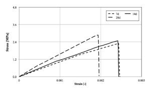
**Figure 7.** Bending stress vs. strain at different aging period (PEG 6 wt%).
