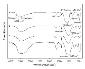
**Figure 1.** (a) MK FTIR spectrum compared with FTIR spectra of GP0 after (b) 7 days (c) 14 days and (d) 28 days.
