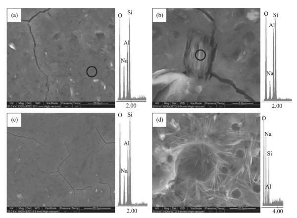
Figure 4. SEM micrograph and EDS analysis. (a) GP0 after 7 days and EDS performed on an reacted area (indicated in circle). (b) nonreacted metakaolin fibrous structure in GP0 after 7 days and EDS analysis. (c) GP0 after 21 days and EDS analysis performed randomly on surface. (d) SEM micrograph of crystals found on air exposed surface and their EDS spectra.
