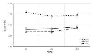
Figure 8. Bending strength vs. aging at different PEG percentages.
