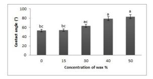
Figure 2. Mean values for contact angle as a function of the carnauba wax percentage in the lipid mixture for the different polymer: lipid ratios. Different lowercase letters mark significantly different mean values.
