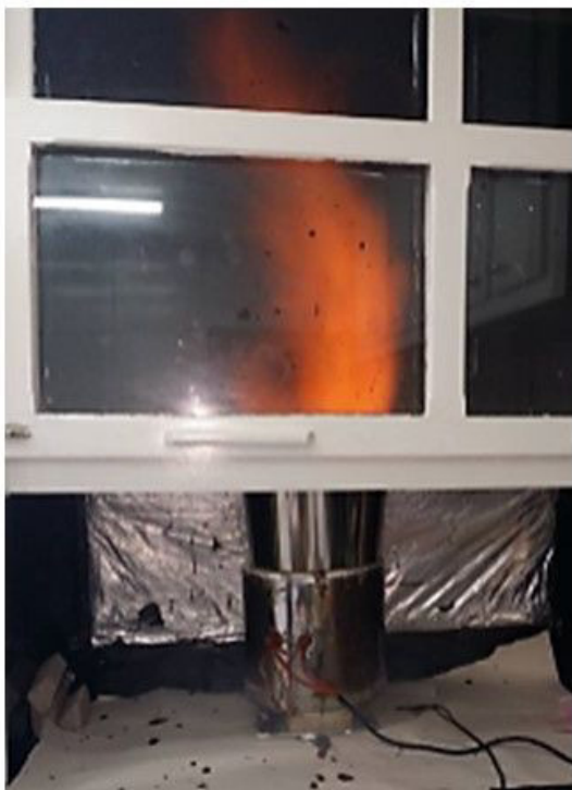
Figure 1. Redox mixture of metal nitrates and fuel on heating in the reactor.
