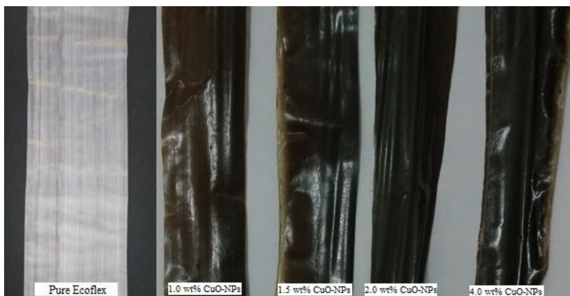
Figure 4. Image of the polymeric obtained films with 1 wt%, 1.5 wt%, 2 wt% and 4 wt% CuO-NPs and of the polymeric obtained films in the absence of CuO-NPs (pure Ecoflex®).
