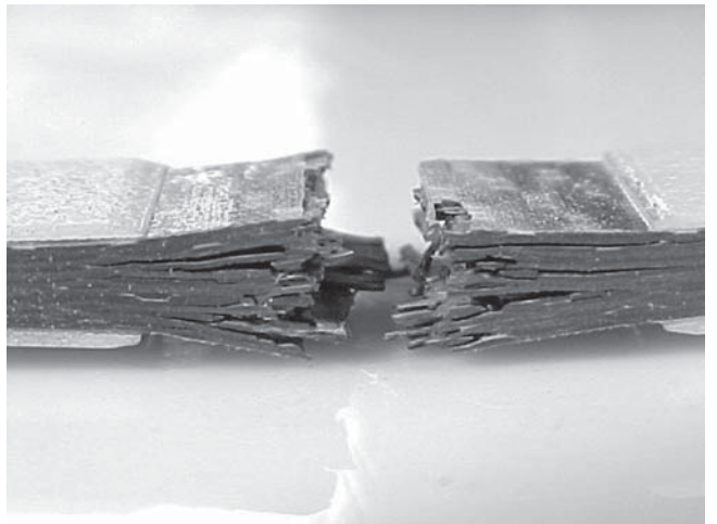
Figure 10. F155/8HS laminate after compression test, showing "axial splitting" fracture.
