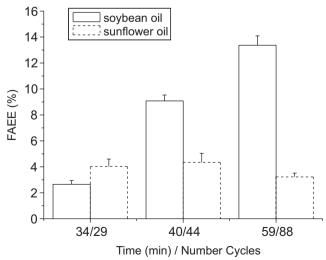
Figure 5. FAEE production by enzymatic transesterification of vegetable oils under MW by power cycling mode (PC) with tert-butanol. Conditions: 60 °C, 3.36% enzyme loading
