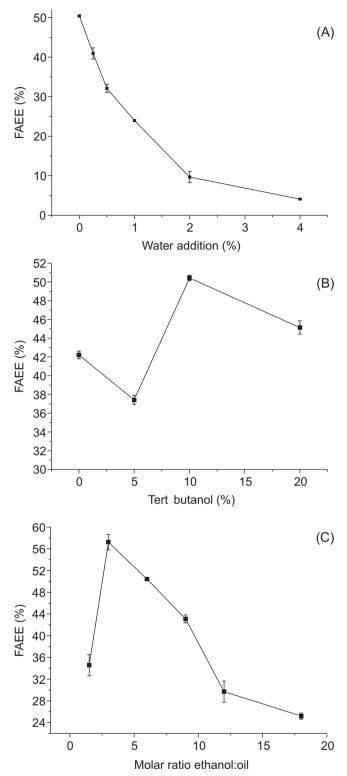
Figure 2. Effect of water addition (A), tert-butanol (B) and molar ratio (C) on the transesterification of soybean oil catalyzed by Novozyme 435 under CH. Conditions: 60 °C, 3.36% enzyme loading
