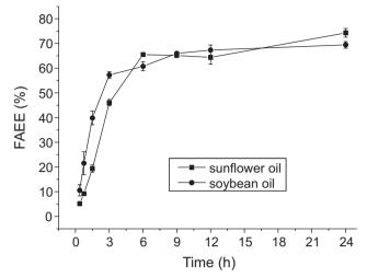
Figure 3. Transesterification progress. Conditions: 60 °C, 1:3 oil-to-ethanol molar ratio, 3.36% enzyme loading, tert-butanol 10%, addition water 0%
