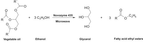
Figure 1. Transesterification of soybean and sunflower oils and ethanol with Novozyme 435 under MW
