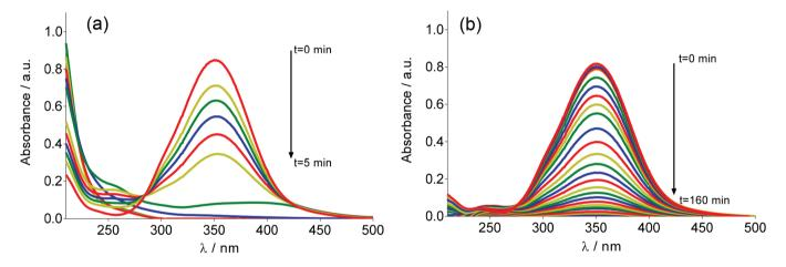
**Figure 1.** Adsorption spectra of aqueous RNO solution  $(2 \times 10^{-5} \text{ mol } L^{-1})$  obtained at different electrolysis-time intervals under galvanostatic conditions, in (a) 0.25 mol  $L^{-1} H_2$ SO<sub>4</sub> and (b) 0.25 mol  $L^{-1} HCO_4$ as supporting electrolytes, at Nb/BDD anode by applying 60 mA cm<sup>-2</sup> at 25 °C
