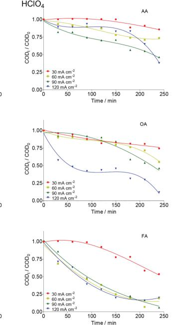
Figure 6. Effect of j on the normalized COD decay as a function of electrolysis time during the EO of AA, OA and FA at Nb/BDD anode surface in 0.25 mol L<sup>-1</sup>  $H_2SO_4$  (left) and 0.25 mol L<sup>-1</sup> HClO<sub>4</sub> (right) applying 30, 60, 90 and 120 mA cm<sup>-2</sup>
