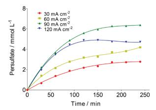
*Figure 4.* Electrogenerated  $S_2O_8^{2-}$  at BDD anode by applying 30, 60, 90 and 120 mA cm<sup>2</sup> during electrolysis in 0.25 mol L<sup>-1</sup> H<sub>2</sub>SO<sub>4</sub> at 25 °C
