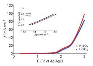
**Figure 5.** Polarization curves and Tafel analysis for Nb/BDD electrode in 0.25 mol  $L^{-1}H_2SO_4$  and 0.25 mol  $L^{-1}HClO_4$  at 50 mV s<sup>-1</sup> at 25°C
