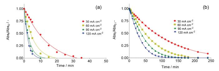
Figure 2. Normalized absorbance decay of RNO solution as consequence of hydroxyl radicals electrogeneration at Nb/BDD anode by applying 30, 60, 90 and 120 mA cm<sup>2</sup> during electrolysis in (a) 0.25 mol  $L^1$  H<sub>2</sub>SO<sub>4</sub> and (b) 0.25 mol  $L^1$  HClO<sub>4</sub> at 25 °C
