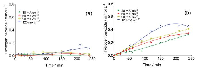
Figure 3. Concentration of electrogenerated  $H_2O_2$  at Nb/BDD surface in (a) 0.25 mol  $L^1H_2SO_4$  and (b) 0.25 mol  $L^1HClO_4$  by applying 30, 60, 90 and 120 mA cm<sup>2</sup> at 25 °C
