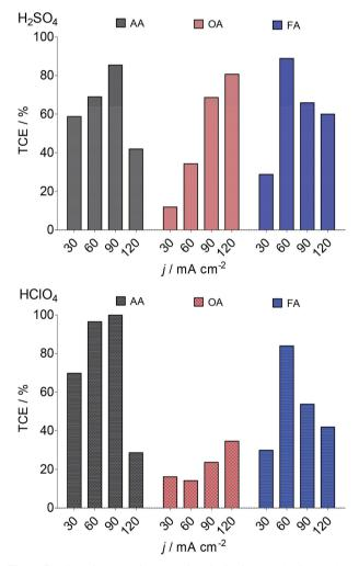
**Figure 7.** TCE values as a function of applied j during EO of AA, OA and FA in 0.25 mol  $L^{-1} H_2SO_4$  and 0.25 mol  $L^{-1} HClO_4$  by using Nb/BDD anode estimated at 240 min of electrolysis
