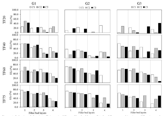
Figure 4. Behavior of cleaning efficiency in different filter bed layers (E<sub>Li</sub>), for different combinations of filtration cycles (C1, C2 and C3), sand granulometries (G1, G2 and G3) and filtration rates (TF20, TF40, TF60 and TF75)
