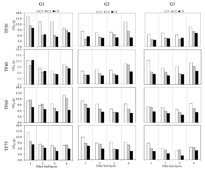
Figure 2. Behavior of mass of solids present in the filter bed after filtration (before backwashing) in different filter bed layers (MS<sub>F</sub>) for different combinations of sand granulometry (G1, G2 and G3), filtration rates (TF20, TF40, TF60 and TF75) and filtration cycles (C1, C2 and C3)
