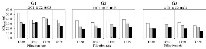
Figure 3. Behavior of total mass of solids present in the filter bed after filtration (before backwashing) (MS<sub>Ftotal</sub>), for different combinations of sand granulometry (G1, G2 and G3), filtration rates (TF20, TF40, TF60 and TF75) and filtration cycles (C1, C2 and C3)
