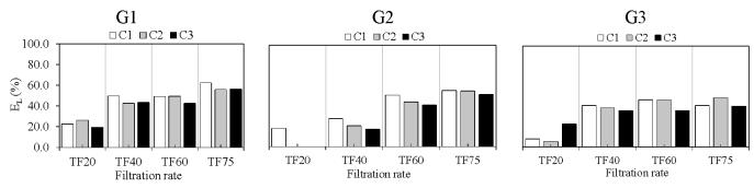
Figure 5. Behavior of cleaning efficiency considering the entire filter bed (E<sub>L</sub>), as a function of different filtration cycles (C1, C2 and C3), sand granulometries (G1, G2 and G3) and filtration rates (TF20, TF40, TF60 and TF75)
