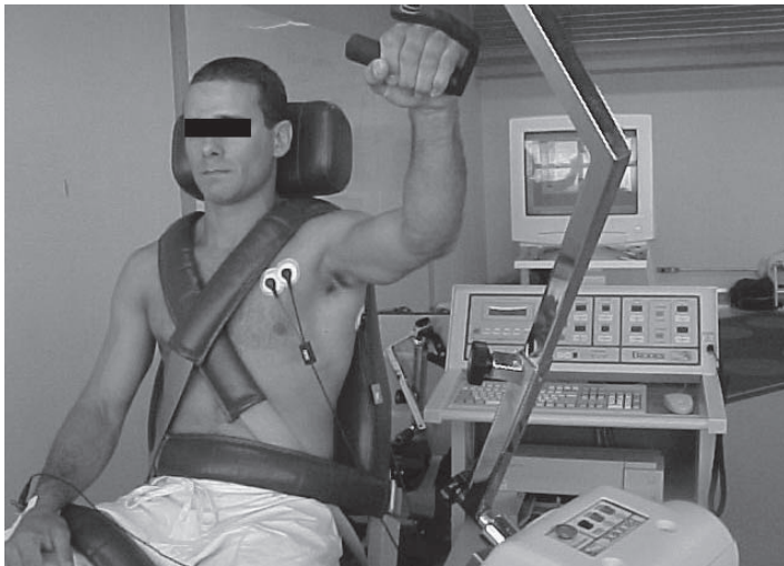
Fig. 1 – Simultaneous collection of the electromyographic signals using an EMG System do Brazil electromyography as well as the torque peak using the Biodes System 3 isokinetic dynamometer
