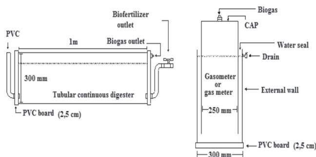
Figure 1 - Schematic representation of a tubular continuous digester of lab bench and gasometer.
