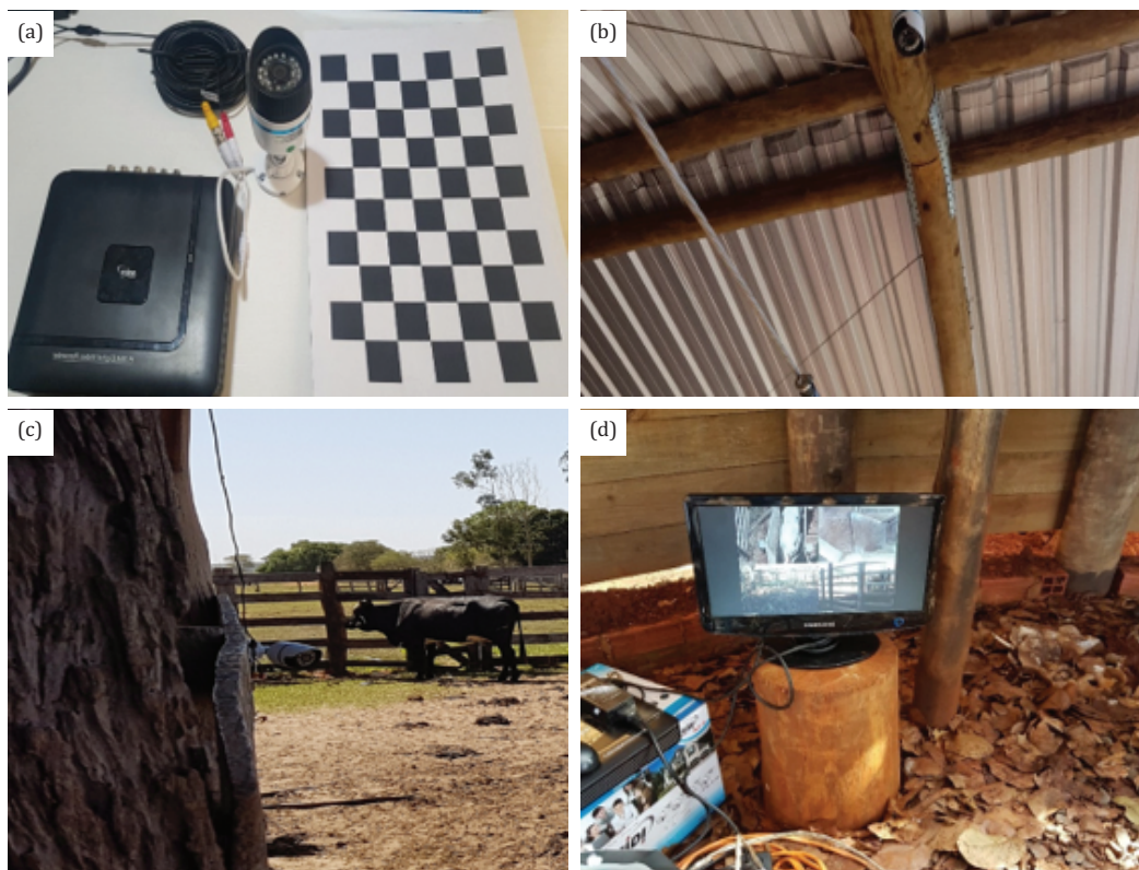
Figure 3 - Image capture equipment (a), camera installed above the squeeze chute for capturing dorsum images (b), camera installed on the fence after the scale for body lateral area image capture (c), and videos recorded on the DVR (d).
