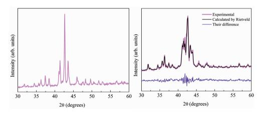
Figure 3 Experimental XRD pattern for the gamma phase.
