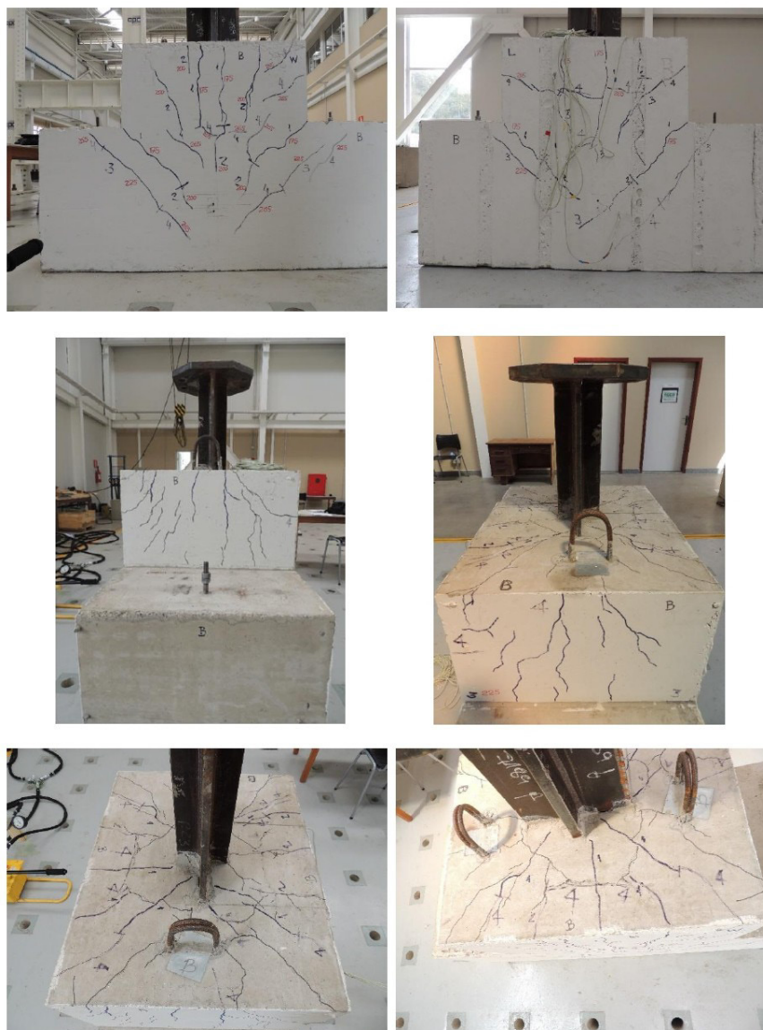
Figure 16. Cracking observed during Specimen B test.
