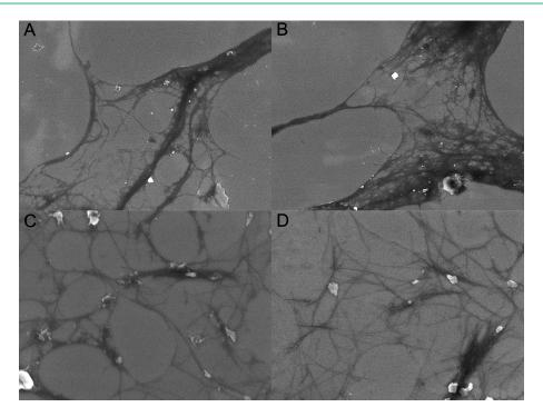
**Figure 6** – A = Scanning electron microscopy images of cellulose nanofiber extracted from peanut peel non-mercerized – CNCNM, (increase of 20,000 times) and B = (increase of 20,000 times) and SEM images of cellulose nanocrystals extracted from peanut peel pre-mercerized (CNCPM), C and D = (increase of 50,000 times).
