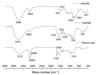
Figure 3 – Furrier Transformed Infrared spectra of peanut peel, cellulose nanocrystals non-mercerized (CNCNM) and, cellulose nanocrystals pre-mercerized (CNCPM).
