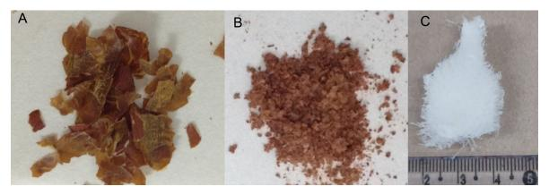
Figure 1 – Images of visual aspect of: A = roasted peanut peel, B = lyophilized cellulose nanocrystals non-mercerized (CNCNM), and C = lyophilized cellulose nanocrystals pre-mercerized (CNCPM).
