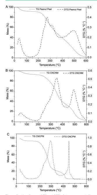
**Figure 2** – A = Curves of TG and DTG of the peanut peel; B = cellulose nanocrystals non-mercerized – CNCNM, and C = cellulose nanocrystals pre-mercerized (CNCPM), in oxidative atmosphere (synthetic air).
