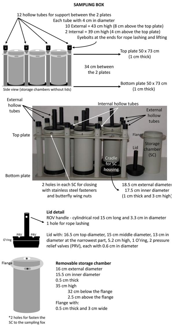
**Figure 2. New sampling box scheme with detail regarding all its components and associated dimensions in detail.**
