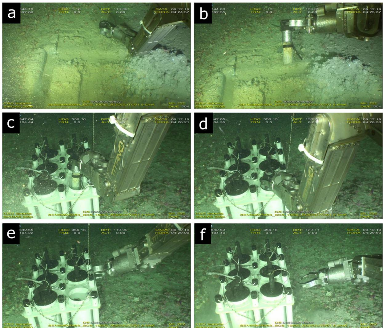
**Figure 4.** Small acrylic push-core being operated by ROV for soft sediment collection. a: ROV pushing the corer against the seafloor, b: ROV pulling the push-core, c-d: push-core being deposited by the ROV into the storage chamber of the sampling box, e: push-core inside the storage chamber, f: storage chamber recently capped by the ROV.
