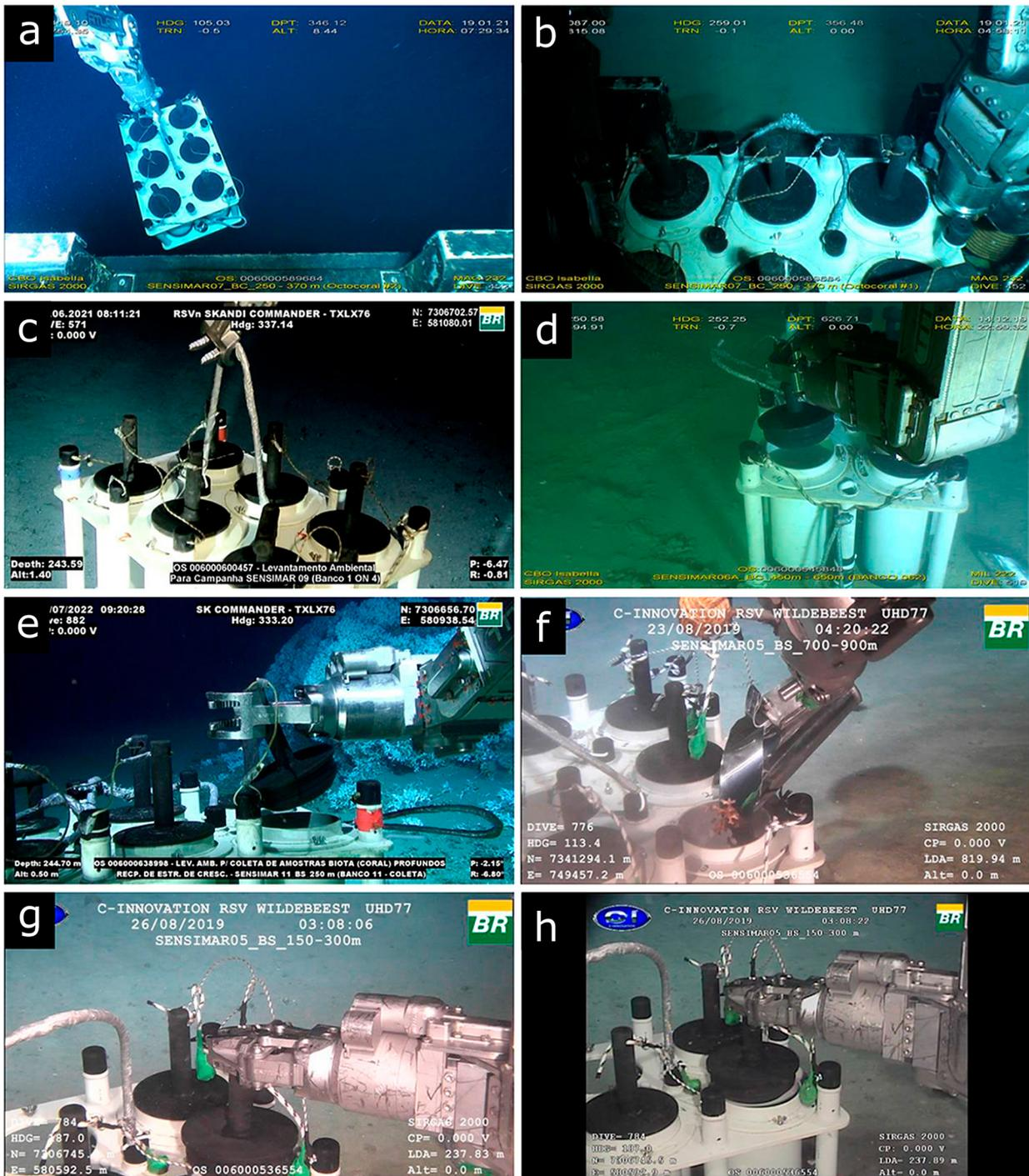
**Figure 3.** New sampling box being operated by different ROVs. a: Sampling box being carried by ROV's 5-function manipulator arm, b: sampling box being carried in the ROV skid/tool drawer, c: sampling box being placed on the seabed by ROV's 7-function manipulator arm, d: ROV uncapping the storage chamber, e: ROV uncapping the storage chamber (in detail), f: ROV pouring biota sampling into the storage chamber, g: ROV capping the storage chamber, h: ROV capping the storage chamber (in detail).
