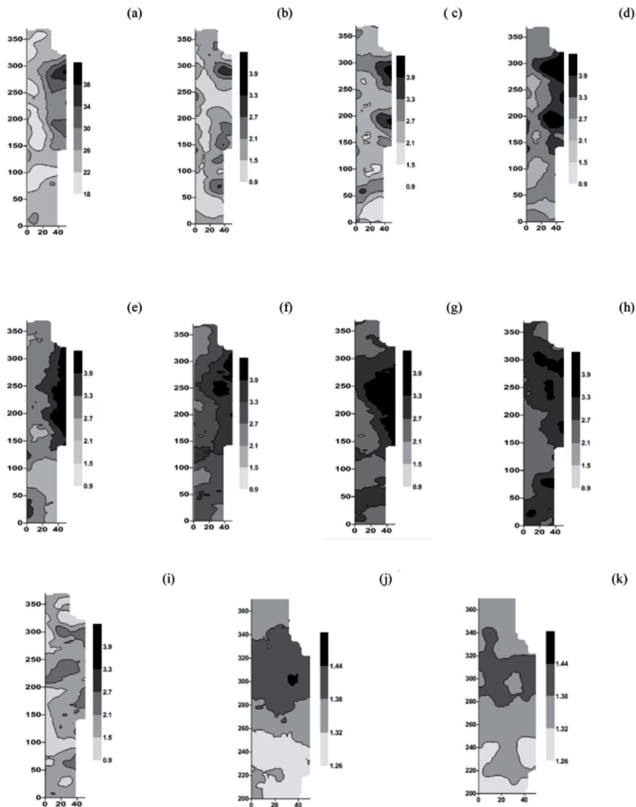
**Figure 5.** Maps for resistance penetration of soil 0.0-0.4 m depth: (a) Strokes of number; (b) Resistance kPa 0.0-0.05 m; (c) Resistance kPa 0.05-0.10 m; (d) Resistance kPa 0.10-0.15 m; (e) Resistance kPa 0.15-0.20 m; (f) Resistance kPa 0.20-0.25 m; (g) Resistance kPa 0.25-0.30 m; (h) Resistance kPa 0.30-0.35 m; (i) Resistance kPa 0.35-0.40 m. Maps for soil density (kg m<sup>-3</sup>): (j) 0.0-0.20 m of the depth; (k) 0.20-0.40 m of the depth.
