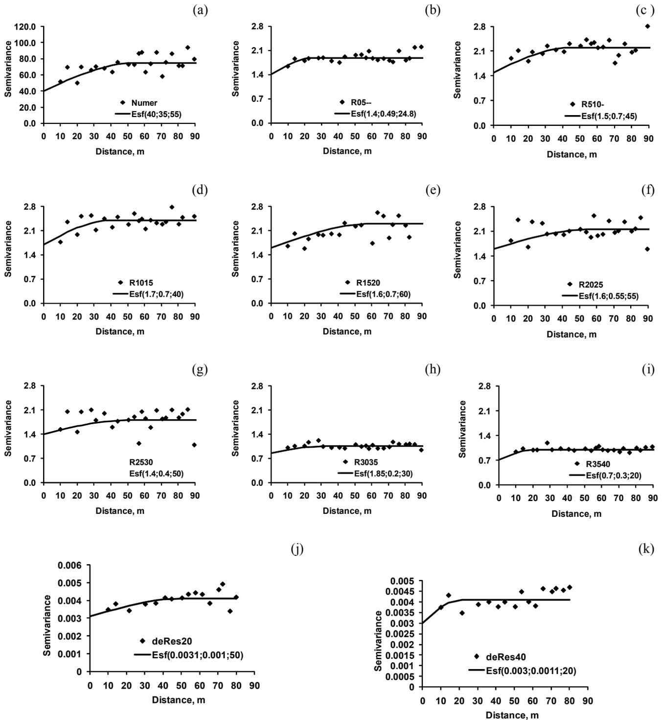
**Figure 2.** Semivariograms for resistance soil penetration 0.0 a 0.40 m of depth: a) Strokes number; b) Resistance kPa 0-0.05 m; c) Resistance kPa 0.05-0.10 m; d) Resistance kPa 0.10-0.15 m; e) Resistance kPa 0.15-0.20 m; f) Resistance kPa 0.20-0.25 m; g) Resistance kPa 0.25-0.30 m; h) Resistance kPa 0.30-0.35 m; i) Resistance kPa 0.35-0.40 m, j) soil density 0.0-0.20 m; k) soil density 0.20-0.40m. Semivariograms for soil density : j) 0.0-0.20 m of the depth; k) 0.2-0.40 m of the depth.
