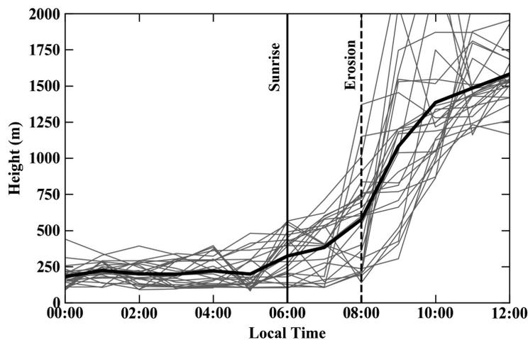
**Figure 3.** Erosion process of the nocturnal boundary layer (NBL) at a central Amazon site during the dry season [Intensive Observation Period 2 (IOP2) of Project GoAmazon2014/5] as measured by Ceilometer. The gray lines represent the measurements for each days of the period. The black line represents period mean. The vertical lines mark sunrise (06:00 LT) and the erosion of the NBL (08:00 LT).
