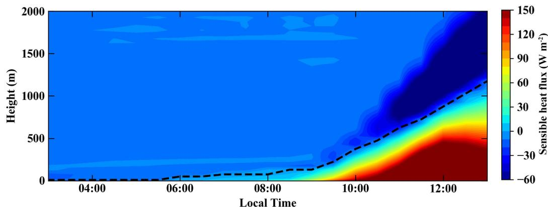
**Figure 4.** Temporal evolution of the sensible heat flux ( $H$ ) ( $\text{W m}^{-2}$ ) profile obtained by the PALM model at a central Amazon site on October 1, 2014. The dashed line represents the height where the flux is zero ( $H = 0$ ). This figure is in color in the electronic version.
