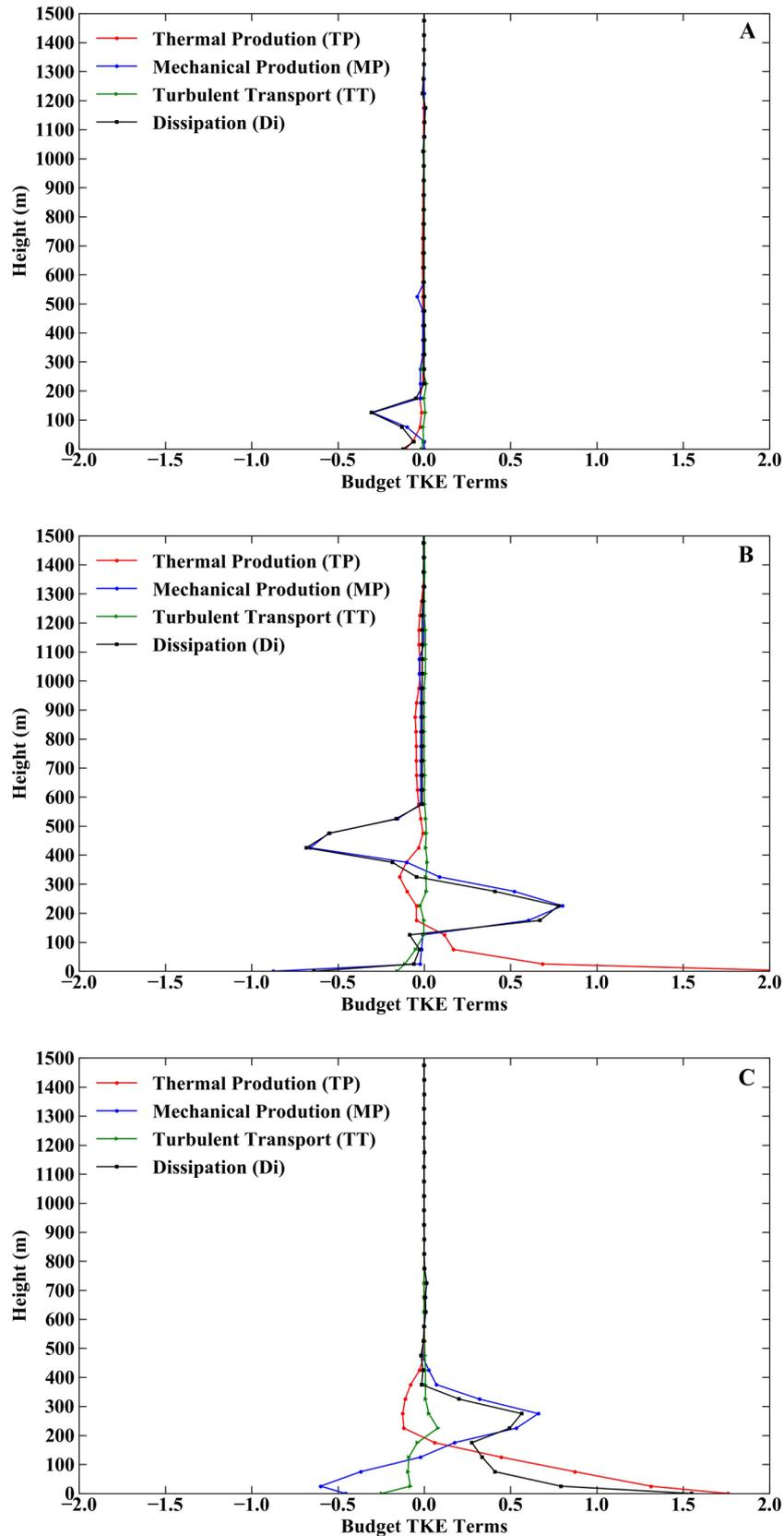
**Figure 6.** Budget of turbulent kinetic energy (TKE) terms at different times of the day (central Amazon local time): A – 04:00 LT; B – 08:00 LT; and C – 10:00 LT. TP = thermal production, MP = mechanical production, TT = turbulent transport, Di = dissipation. This figure is in color in the electronic version.
