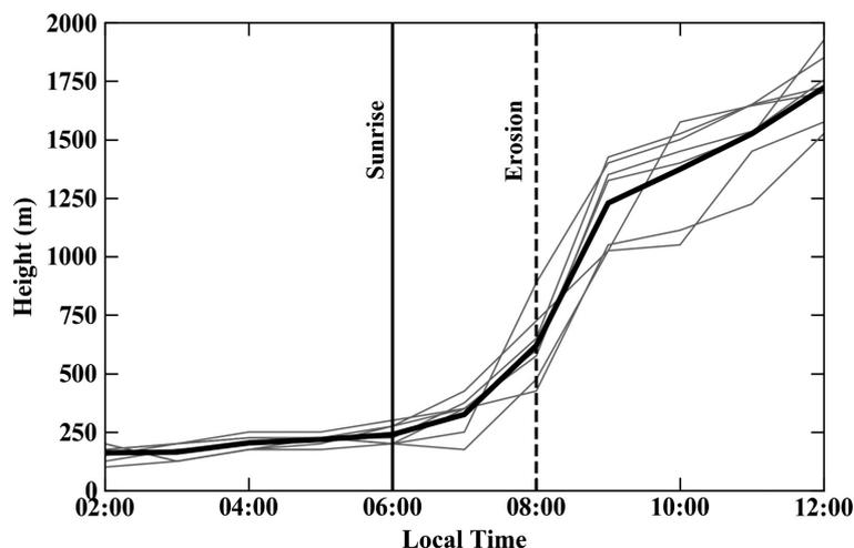
**Figure 7.** Erosion process of the nocturnal boundary layer (NBL) during the dry season at a central Amazon site obtained by PALM. The gray lines represent the simulated days. The black line represents the dry season mean. The vertical lines represent sunrise (06:00 LT) and erosion of the NBL (08:00 LT).
