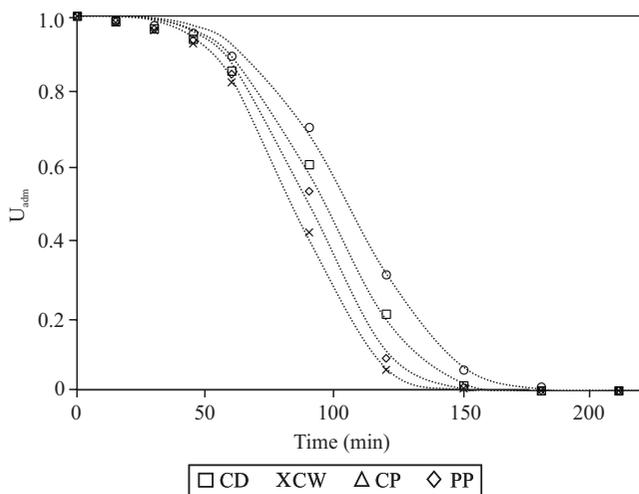
**Figure 1.** Drying curves of beetroot (*Beta vulgaris*) slices subjected to the following pretreatments: CD, dry control; CW, wet control; CP, cellulase pretreatment; and PP, pectinase pretreatment. Dotted lines are adjusted curves of a modified Page model.
