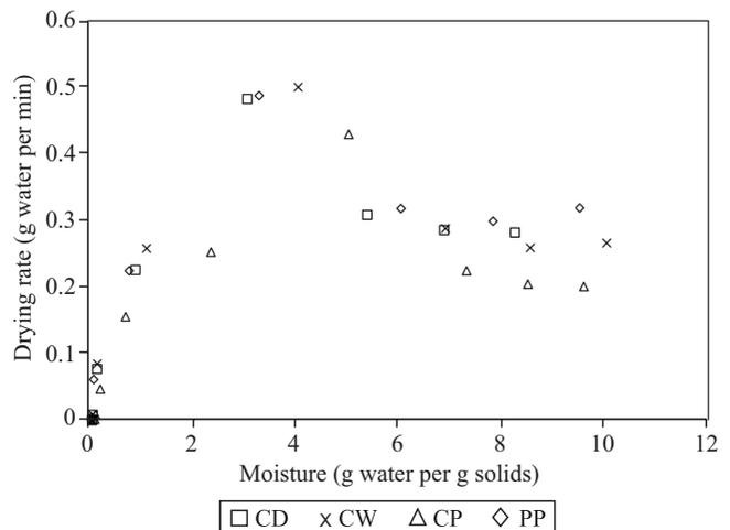
**Figure 2.** Drying rates vs moisture of beetroot (*Beta vulgaris*) slices subjected to the following pretreatments: CD, dry control; CW, wet control; CP, cellulase pretreatment; and PP, pectinase pretreatment.
