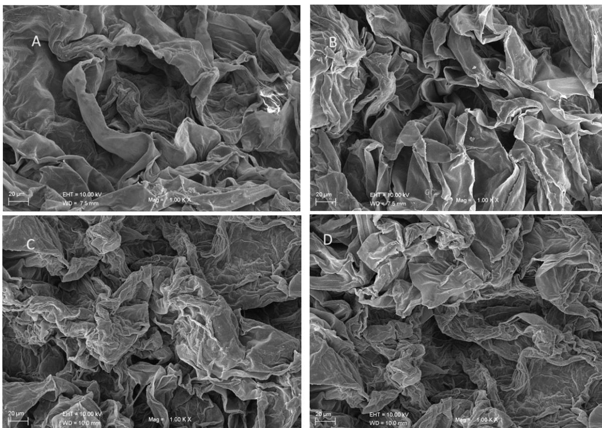
**Figure 3.** Scanning electron microscopy images of beetroot (*Beta vulgaris*) subjected to the following pretreatments: A, dry control (CD); B, wet control (CW); C, pectinase pretreatment (PP); and D, cellulase pretreatment (CP). Magnification: 1,000X.
