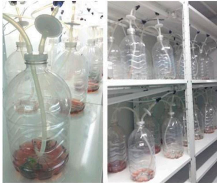
Figure 1. A system of temporary immersion bioreactors in double flasks for multiplication and rooting of 'Pircinque' strawberry explants, on the left, explants in contact with the culture medium and on the right, a view of the complete system, where the liquid medium is in the flask without explants.
