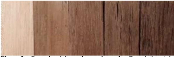
**Figure 2** – Control and thermal treated samples. From left to right: control, 155, 165, 175 and 185 °C.
