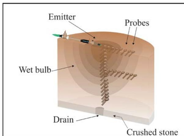
FIGURE 4. Scheme of distribution of TDR probes for determining the movement of the water.
