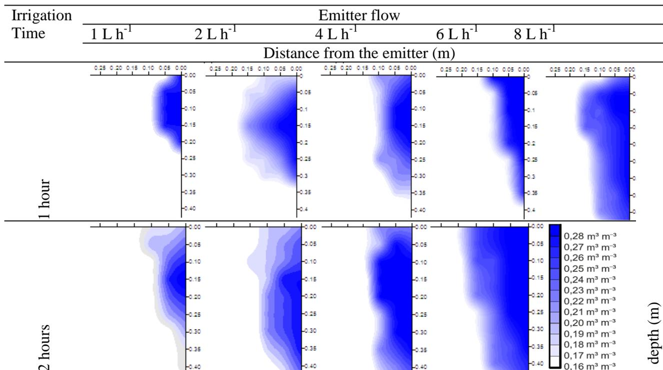
FIGURE 7. Distribution of water for different flow rates up to 0.40 m depth, and emitter placed in the subsurface.
