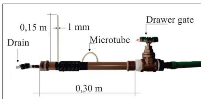
FIGURE 2. Dimensions of emitter built for experimentation.
