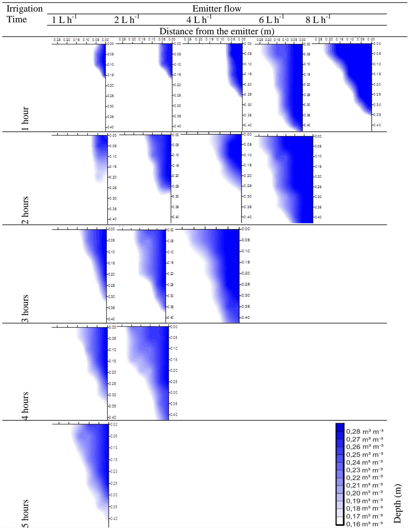
FIGURE 6. Distribution of water for different flow rates up to 0.40 m depth, and emitter placed in the surface.
