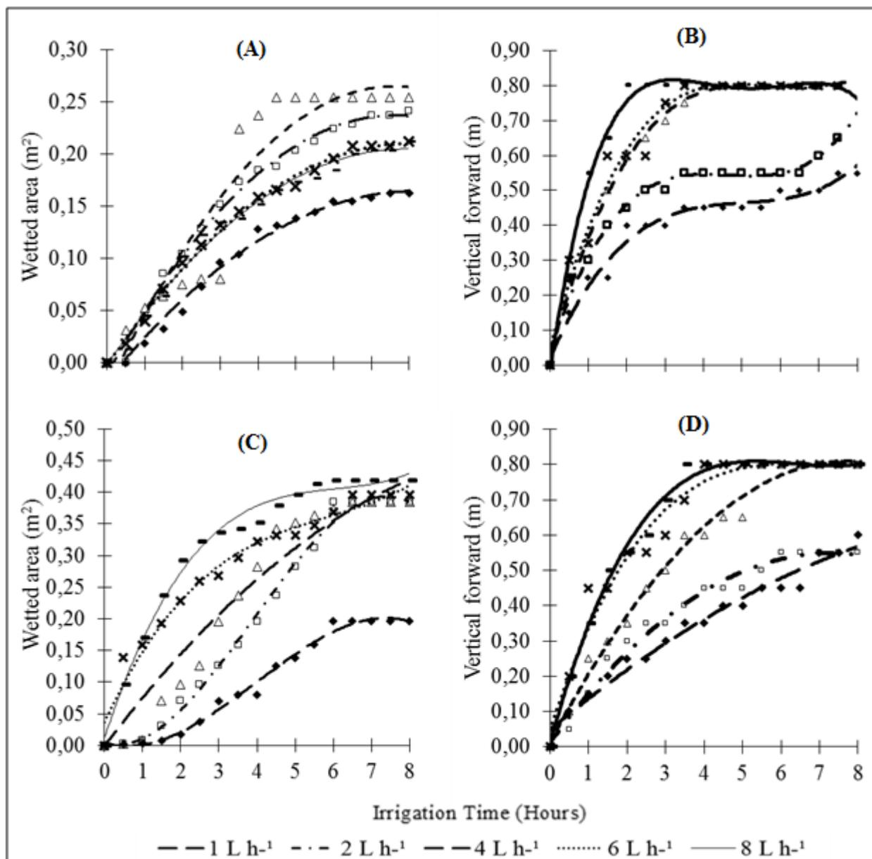
FIGURE 5. Wet area and vertical forward of the front wetting as function of time for irrigation for the emitters at surface (A) and (B) and subsurface (C) and (D), respectively.
