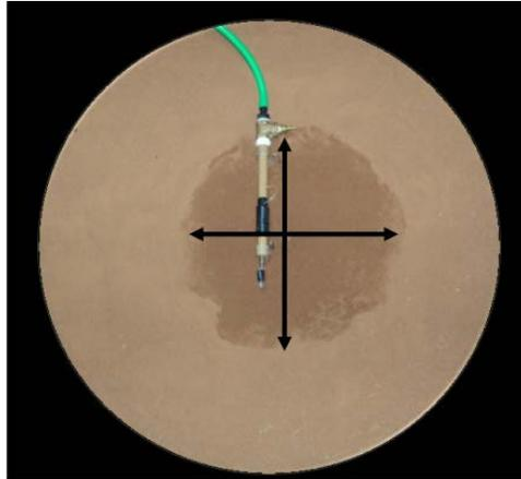
FIGURE 3. Direction representation of the measures, horizontal and vertical determination of the wetted area.
