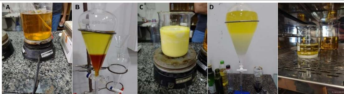
FIGURE 1. Crambe oil and methyl alcohol mixing process (A), separation of glycerin from crambe biodiesel (B), crambe biodiesel washing process (C), biodiesel washing separation (D), biodiesel drying in the greenhouse (E).
