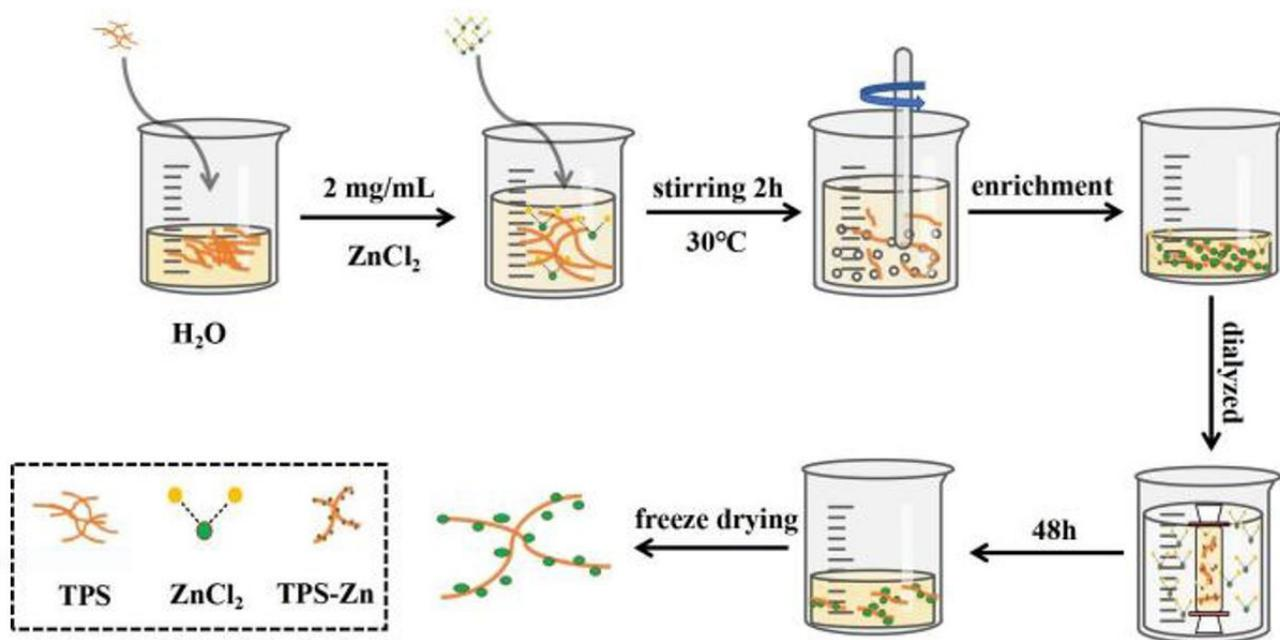
**Figure 1.** Schematic illustration for the preparation of TPS-Zn.
