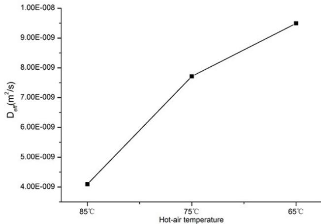
**Figure 4.** Variation of effective moisture diffusivity with drying air temperature.
