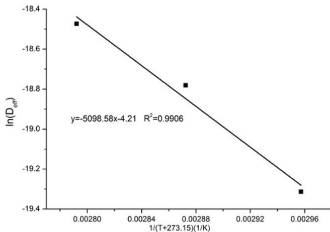
**Figure 5.** Arrhenius-type relationship between  $D_{eff}$  and drying air temperature.
