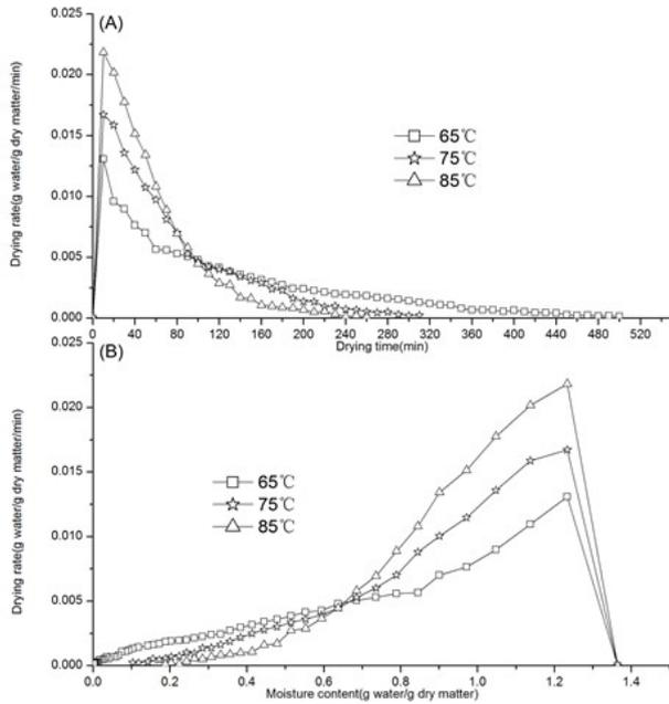
**Figure 2.** Drying rate versus drying time (A) and moisture content (B) of lily scales at different temperatures.
