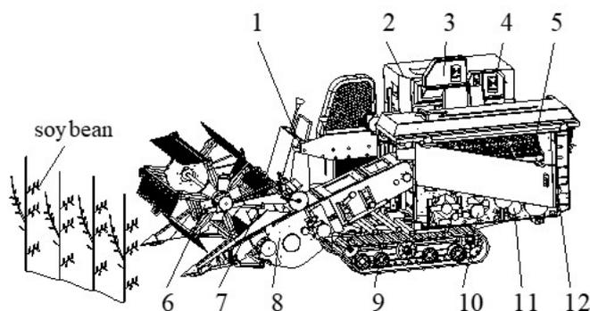
**Figure 1.** Structure diagram of the crawler soybean combine harvester 1. Driver's cab; 2. Grain box; 3. Seed lifter; 4. Re-threshing lifter; 5. Threshing roller; 6. Threshing wheel; 7. header feeding auger; 8. header; 9. Chassis; 10. Horizontal seed spiral conveyor; 11. Horizontal miscellaneous residue spiral conveyor; 12. Cleaning sieve.
