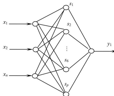
Figure 1. Structure diagram of BP neural network.
