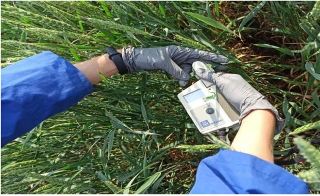
**Figure 6.** Determination of the nitrogen content in the leaves of spring wheat on seed crops with a portable device N-tester, 28.07.2020.
