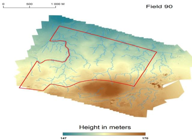
**Figure 4.** Digital elevation model and watercourses for field No. 90.
