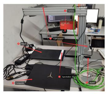
Figure 1. Schematic diagram of hyperspectral imaging system.
