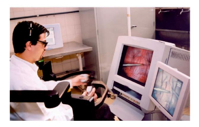
**FIGURE 2** - The main surgeon is in the control console of the Zeus? , geographically apart from the main OR, dissecting the bladder under a three-dimensional image.
