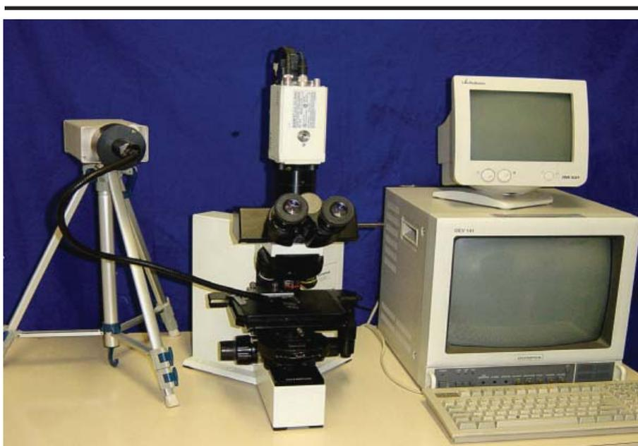
**FIGURE 1** - Stroboscope lamp coupled to the microscope equipped with an image-capturing system
