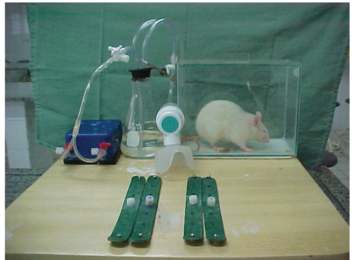
FIGURE 2 - Anesthetic equipment in use, with a rat in the induction chamber and the pediatric inhalation mask.
