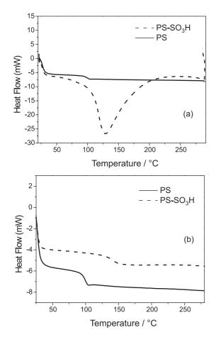
Figure 5. DSC curves for PS and PS-22.0SO3H: (a) first heating run and (b) second heating run.
