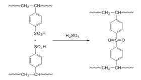
Figure 2. Crosslinking reaction of PS-SO<sub>3</sub>H.
