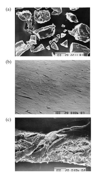
Figure 7. SEM micrographs of (a) powder  $PS-22.0SO_3H$ , (b) film  $PS-22.0SO_3H$  and (c) fractured film  $PS-22.0SO_3H$ .
