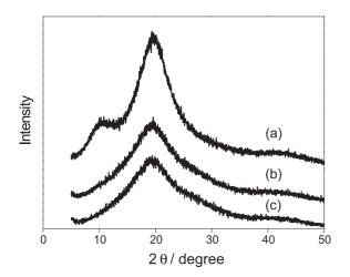
Figure 6. X-ray diffraction patterns of pure PS (a) and (b) PS-22.0SO\_3H and (c) PS-19.7SO\_3H.
