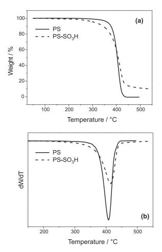
Figure 4. (a) Thermogravimetic curves (10 °C min<sup>-1</sup>, argon) for PS and PS-22.0SO<sub>3</sub>H and (b) DTG curves of samples.
