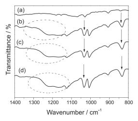
**Figure 3.** Infrared spectra of (a) PS, (b) PS- $18.0SO_3H$ , (c) PS- $40.0SO_3H$  and (d) PS- $22.0SO_3H$ . The arrows designate the absorbances due to sulfonation.
