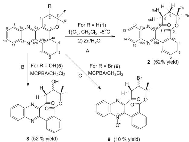
**Figure 2.** Oxidation of phenazines. A: ozonization of lapazine 1 furnishing 2; B: oxidation of 5 furnishing 8; C: oxidation of 6 furnishing 9.
