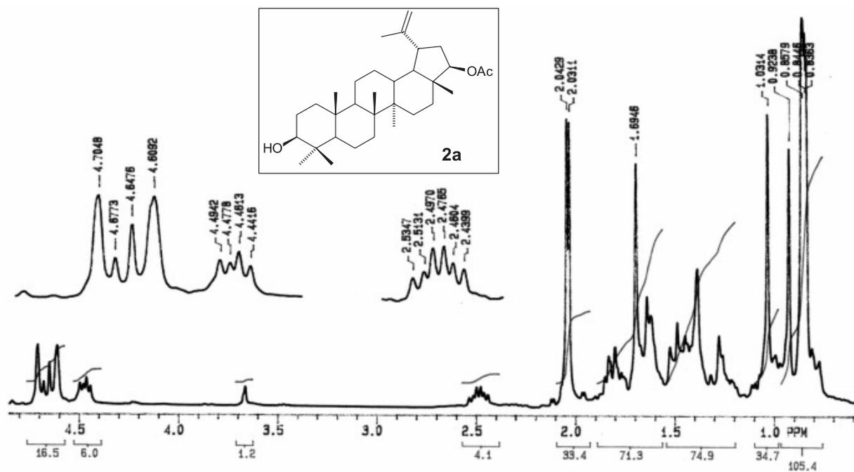
Figure S9.  $^1\text{H NMR}$  of compound 2a [300 MHz,  $\text{CDCl}_3$ ,  $\delta$  (ppm)].
