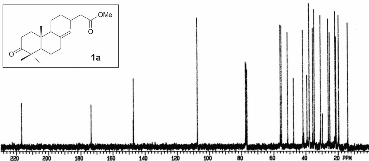
Figure S2.  $^{13}\text{C}$  NMR of compound **1a** [75 MHz,  $\text{CDCl}_3$ ,  $\delta$  (ppm)].
