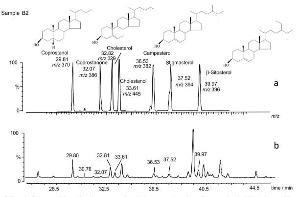
Figure 3. Example of (a) mass and (b) total ion chromatograms of steroids in representative surface sediment sampling site B2 in the Paranaguá Estuarine System.
