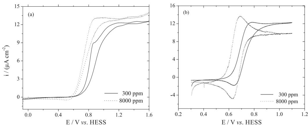
**Figure 3.** Cyclic voltammograms recorded in  $1 \times 10^{-3} \text{ mol L}^{-1} \text{ K}_4[\text{Fe}(\text{CN})_6] + 0.5 \text{ mol L}^{-1} \text{ H}_2\text{SO}_4$  at BDD electrodes (a) anodically and (b) cathodically pre-polarized at  $\pm 10 \text{ C cm}^{-2}$  using  $\pm 1 \text{ A cm}^{-2}$ ,  $v = 0.5 \text{ mV s}^{-1}$ .
