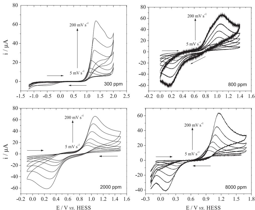
**Figure 2.** Cyclic voltammograms recorded in  $1 \times 10^{-3} \text{ mol L}^{-1} \text{ K}_4[\text{Fe}(\text{CN})_6] + 0.5 \text{ mol L}^{-1} \text{ H}_2\text{SO}_4$  at BDD electrodes anodically pre-polarized at  $10 \text{ C cm}^{-2}$  using  $1 \text{ A cm}^{-2}$ . Doping levels and scan rates are indicated in each figure.
