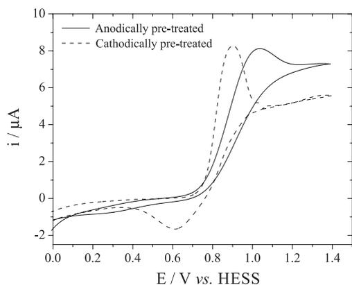
**Figure 5.** Cyclic voltammograms recorded in  $1 \times 10^{-3} \text{ mol L}^{-1}$  hydroquinone +  $0.5 \text{ mol L}^{-1} \text{ H}_2\text{SO}_4$  on 800 ppm BDD electrodes anodically (solid curve) and cathodically (dashed curve) pre-polarized at  $\pm 10 \text{ C cm}^{-2}$  using  $\pm 1 \text{ A cm}^{-2}$ ,  $v = 0.5 \text{ mV s}^{-1}$ .
