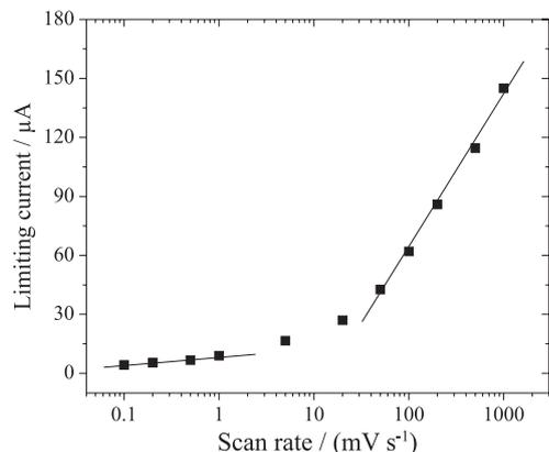
**Figure 4.** Dependency of current on the scan rate for the oxidation of  $1 \times 10^{-3} \text{ mol L}^{-1} \text{ K}_4[\text{Fe}(\text{CN})_6]$  without supporting electrolyte recorded at 800 ppm BDD electrodes pre-polarized at  $10 \text{ C cm}^{-2}$  using  $1 \text{ A cm}^{-2}$ .
