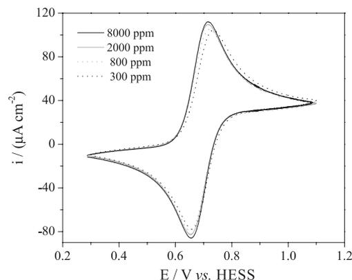
**Figure 1.** Cyclic voltammograms recorded in  $1 \times 10^{-3} \text{ mol L}^{-1} \text{ K}_4[\text{Fe}(\text{CN})_6]$  +  $0.5 \text{ mol L}^{-1} \text{ H}_2\text{SO}_4$  at BDD electrodes cathodically pre-polarized at  $-10 \text{ C cm}^{-2}$  using  $-1 \text{ A cm}^{-2}$ ,  $\nu = 50 \text{ mV s}^{-1}$ .
