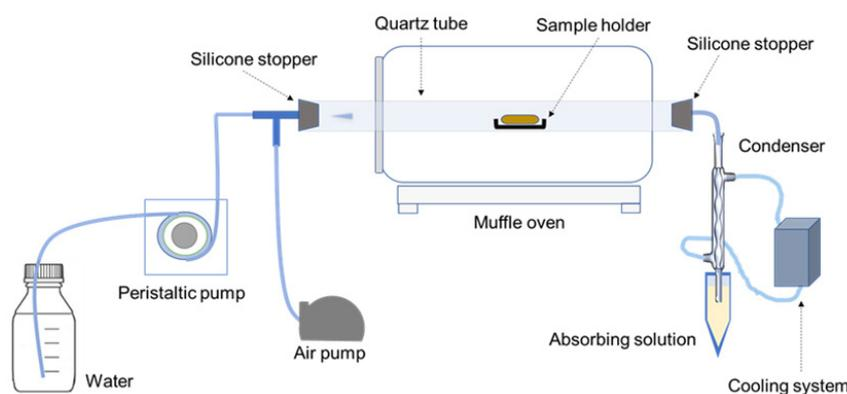
**Figure 1.** Schematic representation of the lab-made pyrohydrolysis system. Quartz tube (17 mm i.d., 400 mm length); alumina sample holder (55 mm length, 10 mm width and 6 mm depth).
