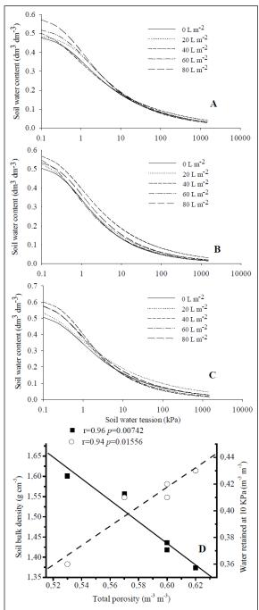
Figure 2 - Water retention curves at 210 (A) 570 (B) and 720 (C) days after the distribution of sawdust on the soil surface. Correlation between soil bulk density, total porosity and water content retained at 10KPa (D). r, Pearson correlation coefficient, p, probability by T test.
