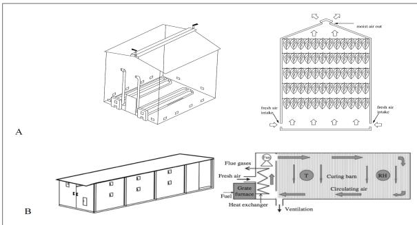
Figure 1 - A: traditional curing unit (masonry); B: air-forced curing unity. Source: C: adapted from TIPPAYAWONG et al. (2004), and D: XIAO et al. (2015).
