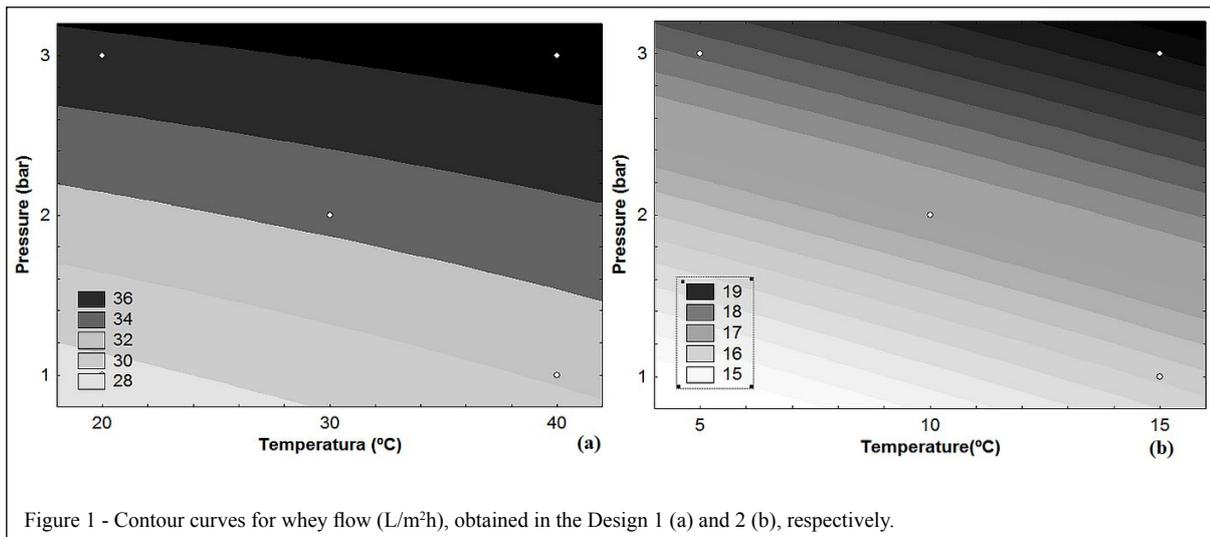
Figure 1 - Contour curves for whey flow (L/m<sup>2</sup>h), obtained in the Design 1 (a) and 2 (b), respectively.
