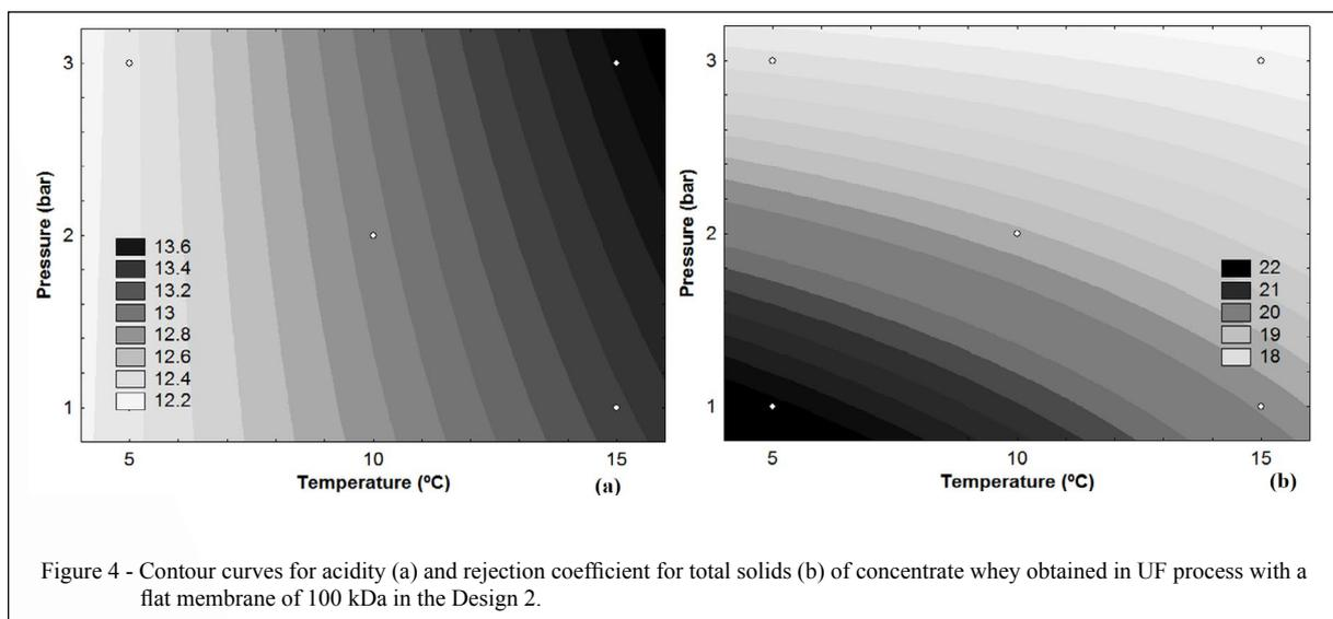
Figure 4 - Contour curves for acidity (a) and rejection coefficient for total solids (b) of concentrate whey obtained in UF process with a flat membrane of  $100\text{ kDa}$  in the Design 2.
