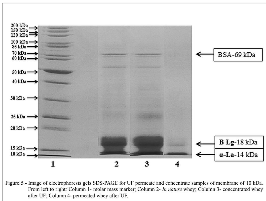
image of the electrophoresis gel. It is observed in the electrophoresis gel that the concentrate sample shows a weak signal for both proteins,  $\beta$ -Lg ( $\beta$ -lactoglobulin of 18.3kDa) and  $\alpha$ -La ( $\alpha$ -lactalbumin of 14.2kDa), indicating that the two proteins are in the concentrate the membrane, since the membrane was 10kDa, thus retaining proteins of molecular weight greater than 10kDa. For the permeated fraction it is not noted a band BSA (69kDa).
