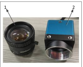
Figure 1 - The physical picture of the camera and lens (1. M1224-MPW2 lens, 2. MER-132-43U3C-L camera).
