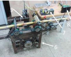
Figure 2 - Experiment platform for detection system of recognition and positioning of sugarcane node. (1. Operation control panel, 2. Image acquisition card, 3. DC power supply, 4. PC host, 5. LabVIEW Inspection System Interface, 6. Conveying mechanism, 7. PLC, 8. Stepper motor driver, 9. Camera holder).
