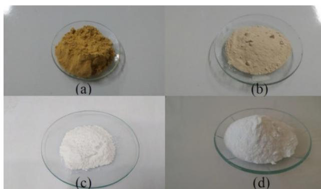
Figure 2: Images of samples: a) Chocolate clay; b) modified Chocolate clay; c) CTAB-MCM-41 (Adsorbent 1); and d) MCM-41 (Adsorbent 2).
