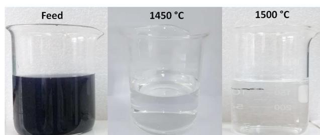
Figure 10: Images of textile effluent before and after treatment with SiC hollow fiber membrane sintered at 1450 and 1500 °C.
